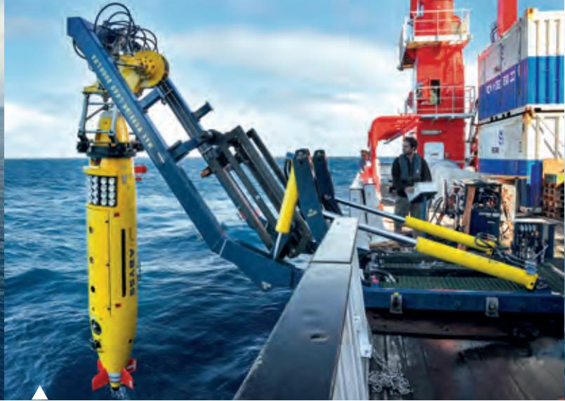
**Deploying AUV ABYSS from board of SONNE.**
