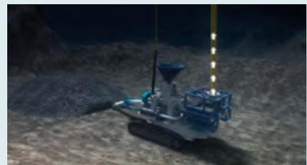
3: The collector collects the broken ores and pumps them via the riser up to the mining vessel.
