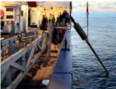
**Gravity corers** are long steel tubes that are lowered vertically into the water. Equipped with weights of several tons, they penetrate up to 20 metres into the seabed and are retrieved to the ship together with the enclosed sediment. Photo: Elger Esser
