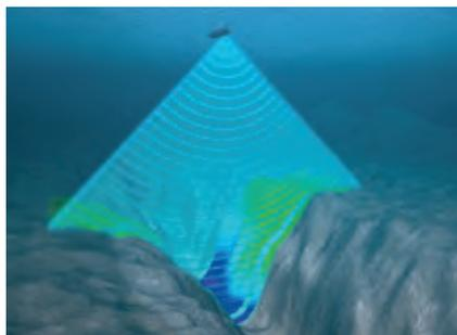
**Ship-based echo sounders** can generate several hundred individual fan segments that scan the seabed perpendicular to the ship's direction of travel in high resolution. Illustration: Wärtsilä ELAC Nautik
