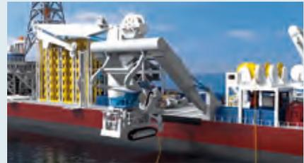
1: Crawlers are released from the mining vessel, which also contains the extraction system and ore storage tanks.
