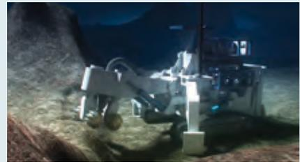
2: The rock cutter is used to break up the massive sulphides on the seabed.
