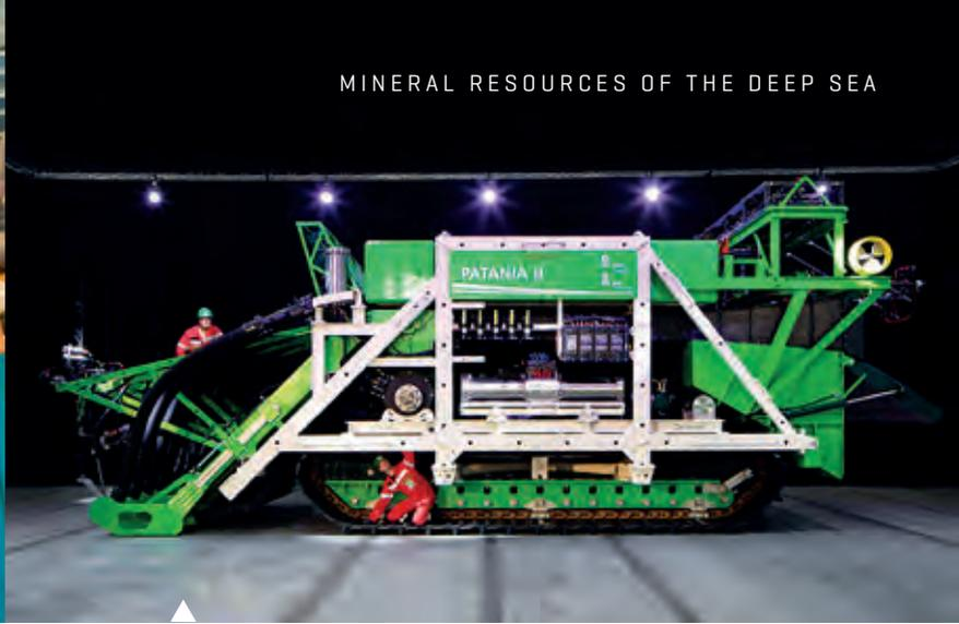
**Prototype collector Patania II of the Belgian company DEME-GSR.**
