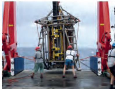
**Rockdrill 2**, a drilling rig of the British Geological Survey, is capable of drilling through hard rock down to 15 metres and is deployed directly at the seabed. Here, the core is drilled in 10 1.5-meter long sections. Source: GEOMAR
