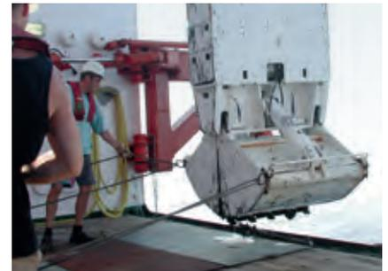
**Video-guided grabs** are equipped with a camera inside that sends real-time videos to the ship via a deep-sea cable. This allows the shovels to be closed in a controlled manner and rock samples to be taken. Photo: Sven Petersen/GEOMAR
