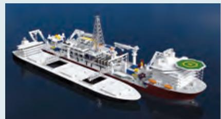
5: The massive sulphides are transferred to a transport vessel which brings the ores ashore for further processing. Picture series: © Nautilus Minerals
