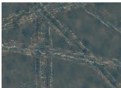
In 1989, during the DISCOL project, researchers towed a plough-harrow 78 times across the abyssal seafloor. Using the ABYSS autonomous underwater vehicle, the researchers were able to produce high-resolution maps that show the precise location of the tracks after 26 years. Source: GEOMAR
