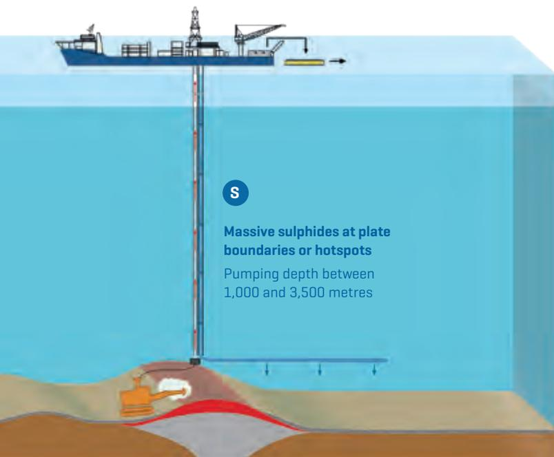
**The deep-sea mining process using the planned exploitation of massive sulphides off Papua New Guinea as an example.**
